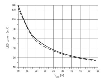
EM converterLED BASIC 203 MH/LiFePO4 50V Article number: 89800576 NiMH battery, 3.6 V battery voltage 810 – 870 mA battery discharge current (tolerance) LiFePO, battery, 3.2 V battery voltage
