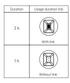
Emergency lighting LED driver supplied with duration link in 3 hours position.
