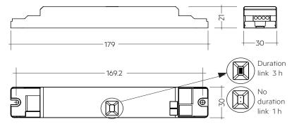
Note: LED driver supplied with duration link in 3 hours position. Remove duration link for 1 hour duration. Duration link must be set before battery and mains connection.
