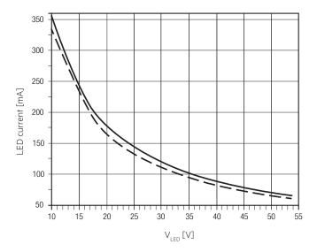
LED current at nominal battery voltage and min. battery discharge current
