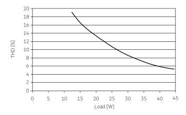
100 % load corresponds to the max. output power (full load) according to the table on page 2.
