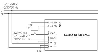
Device with loop through wiring function.
